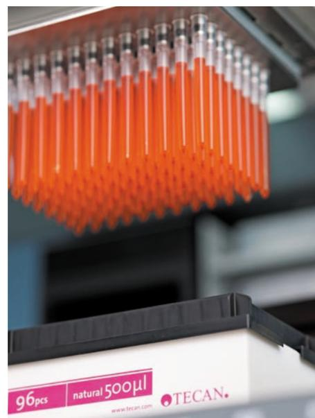
With the Extended Volume Adapter (EVA) the 384-ch. head can pipette up to 500 µl in the 96 well format.
