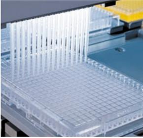
The 384-ch. head pipetting with a column of 16 tips.
