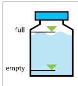
Liquid level detection (LLD) system to monitor bottle fill levels
