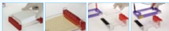
After pouring gel, the 96 well comb is inserted and the gel is allowed to set
