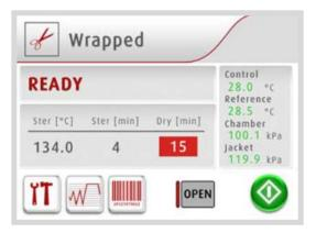
The 7-inch touch screen gives easy access to all control features for operating the autoclave. With technician level password access there are further features available for maintenance, calibration and checking the autoclave.
