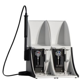
Reagent dispenser with heating and stirring enhances application flexibility: Spark injectors offer a heating and stirring option for reagent storage. This is especially beneficial for cell-based applications, minimizing cold shock caused by reagent addition and enabling automated dispensing of viable cells within the reader.
